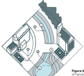
**Figure 55:** Diagram showing the best use of harvesting water systems rain garden, swales, permeable paving, green roofs
