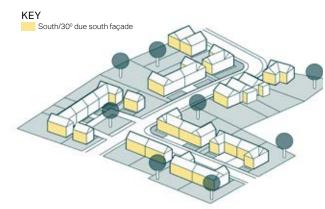
Figure 64: Elevations that would benefit from passive solar gain
