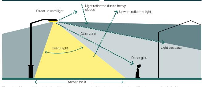
Figure 54: Diagram to illustrate the different components of light pollution and what 'good' lighting means for dark skies.
