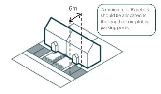
**Figure 39:** Illustrative diagram showing an indicative layout and minimum dimensions of on-plot front parking.
