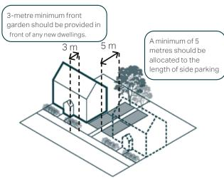
**Figure 38:** Illustrative diagram showing the indicative layout of and minimum dimensions of on-plot side parking, parking bays should be set slightly behind main building frontage to minimise visual impact on streetscapes.
