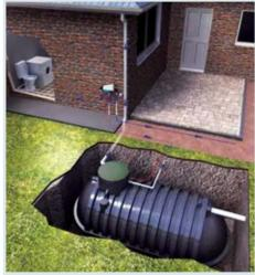
**Figure 61:** Example of an underground water tank in relationship with the building (Source: https://handymantips.org/about-underground-water-tanks/)
