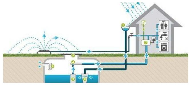
**Figure 58:** Diagram illustrating rainwater harvesting systems that could be integrated into open space and residential developments.
