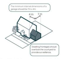
Figure 31: Illustrative diagrams showing the indicative layout of garage parking.
